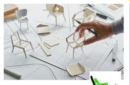
Furniture Design Working with natural wood and timber products for the finished product, a designer will often use paper and board to produce scale models which are quick and comparatively inexpensive to create. Designers use early modelling to: • ensure the product is suitable for use (anthropometrics); • calculate the amount of material required; • research joining solutions; • check structural strength; • check the overall style.
