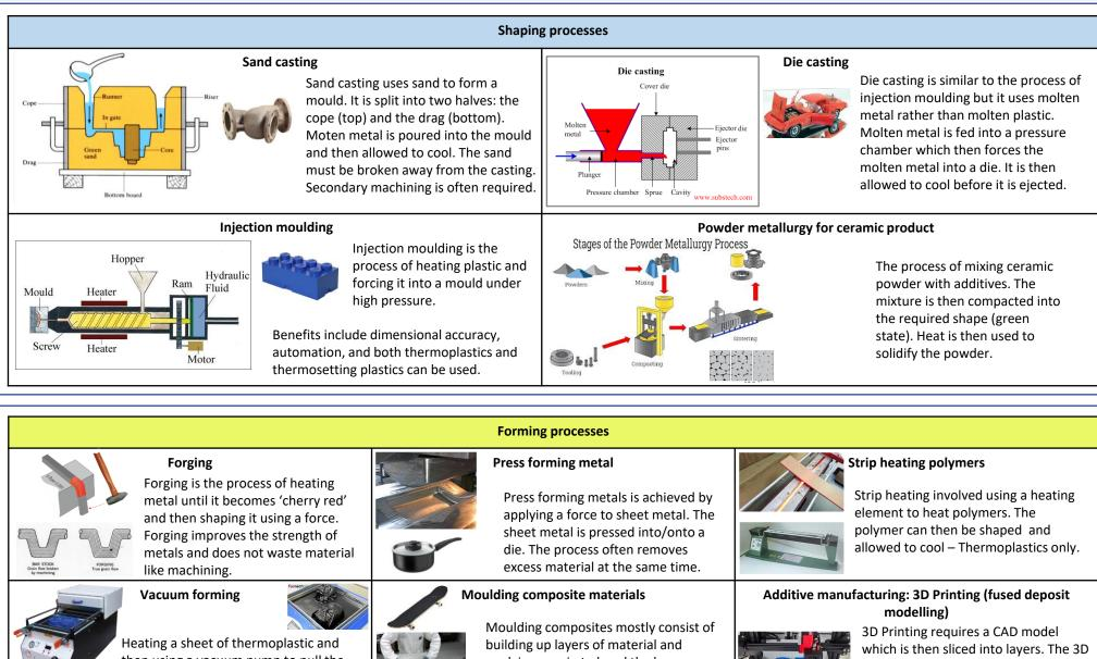
then using a vacuum pump to pull the softened polymer over a mould. Moulds must have a draft angle. Moulding composites mostly consist of building up layers of material and applying a resin to bond the layers together. Moulds in the desired shape are used to form the composite.
