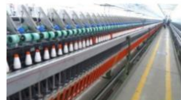
This giant machine spins all the fibres into yarn, ready for weaving.
