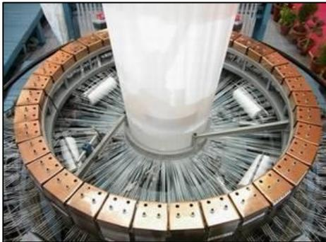
This is a type of loom that is making knitted fabric that is in the shape of a tube. This could be used to make the body of a t-shirt, the arms and neck hole would be attached separately.
